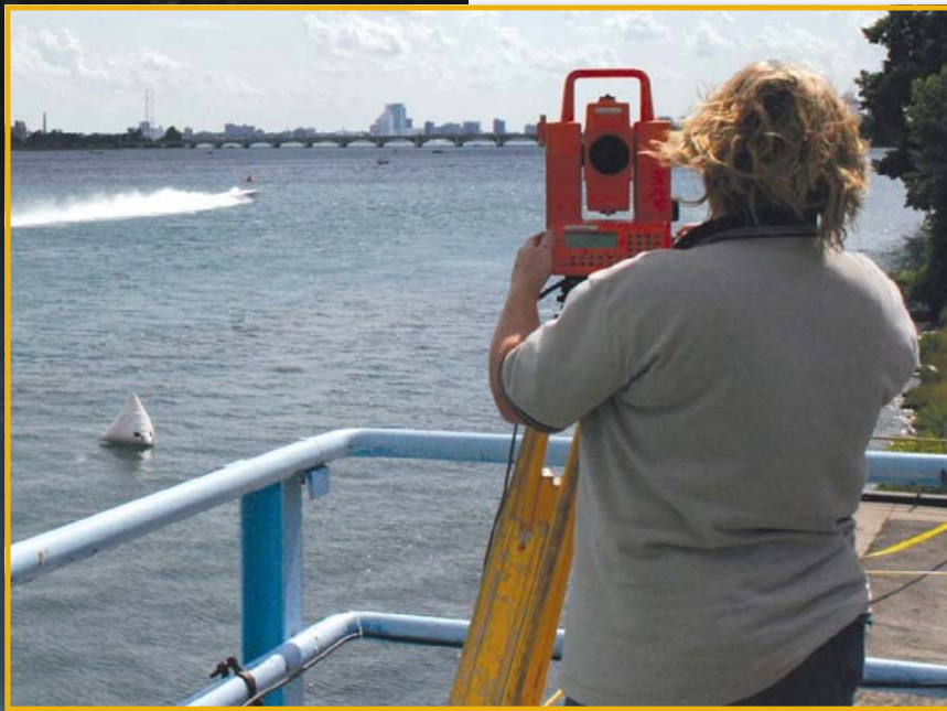
Karol Grove, PS, uses a Trimble Geodimeter 610 Pro robotic instrument to control an onshore survey station during the race. Photo by Reed Zapf.
